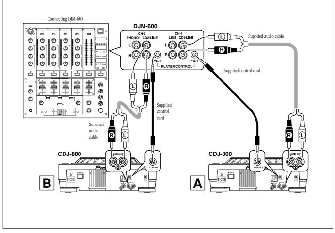
• Connections for the DJM-300 and DJM-500 are similar; use the supplied audio cables to connect the mixer's CD1 jacks to Player A, and CD2 jacks to Player B. When using the DJM-3000, Player A is connected to LINE 1 of CH-1, and Player B is connected to LINE 3 of CH-2.
